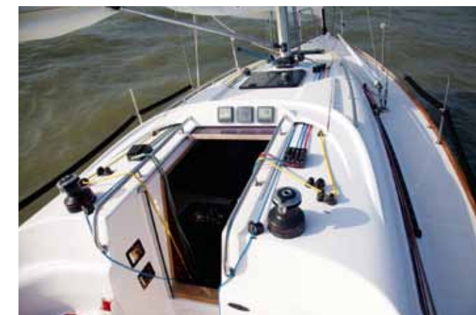
Lines are led aft under removable garages on the coachroof in a layout that's simple and efficient. The kicker and pole downhaul are split to both sides
