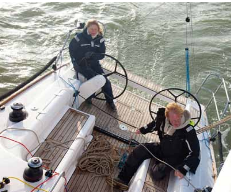
Twin wheels immediately abaft the mainsheet work well for short-handed sailing. Foot-braces are offered and are most definitely needed
