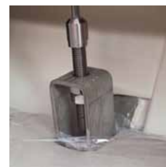
Tie-bars are linked to the stainless steel frame bonded into the bottom of the hull that distributes the loads from the rig and keel
